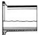
14WLMPT Tank Welding Spud (Light)
